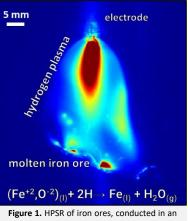
EAF filed with Ar-10% $H_2$  gas mixture. Thermal gradients were captured by special set of lenses [5].
