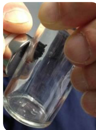
The magnet attracts the carbone spheres against the glass wall of the vial
