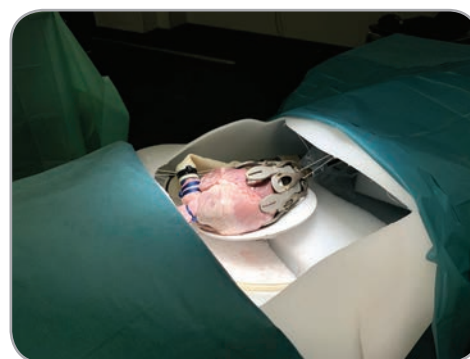
Exoskeleton placed on an explanted porcine heart and simulated in the EXOHEART simulator designed by the consortium
